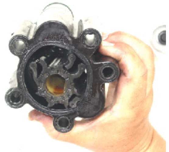
No wonder the mimosas were lumpy —The water pump housing containing Impulse's disintegrated impeller, which caused the starboard engine and its owner to overheat.
